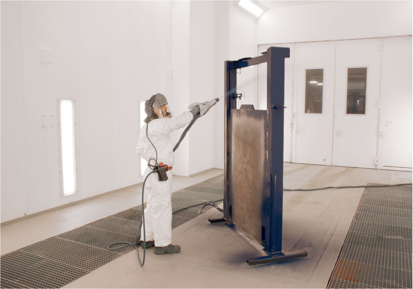
Ideal working environment. The paint mist is reliably extracted and paint vapours are only hardly noticeable during operation.
