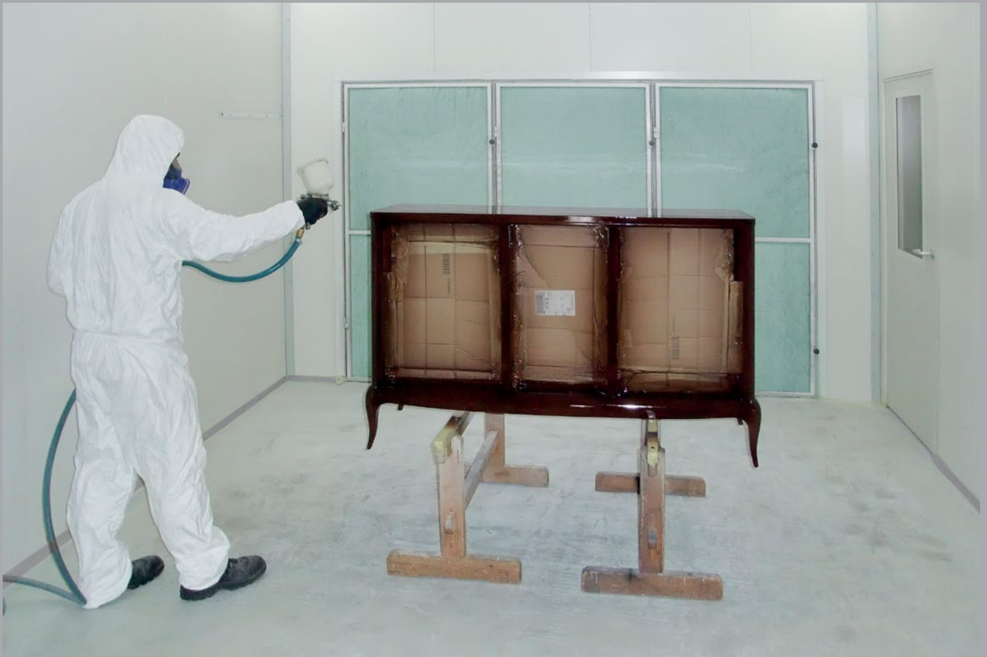
Compact paint booth with integrated drying function in a modern joinery operation.
